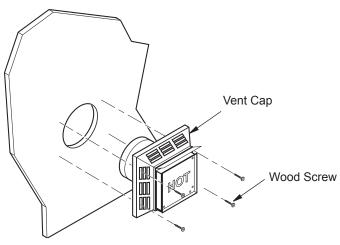
Figure 10 - Installing Horizontal Vent Cap (Noncombustible Exterior)
